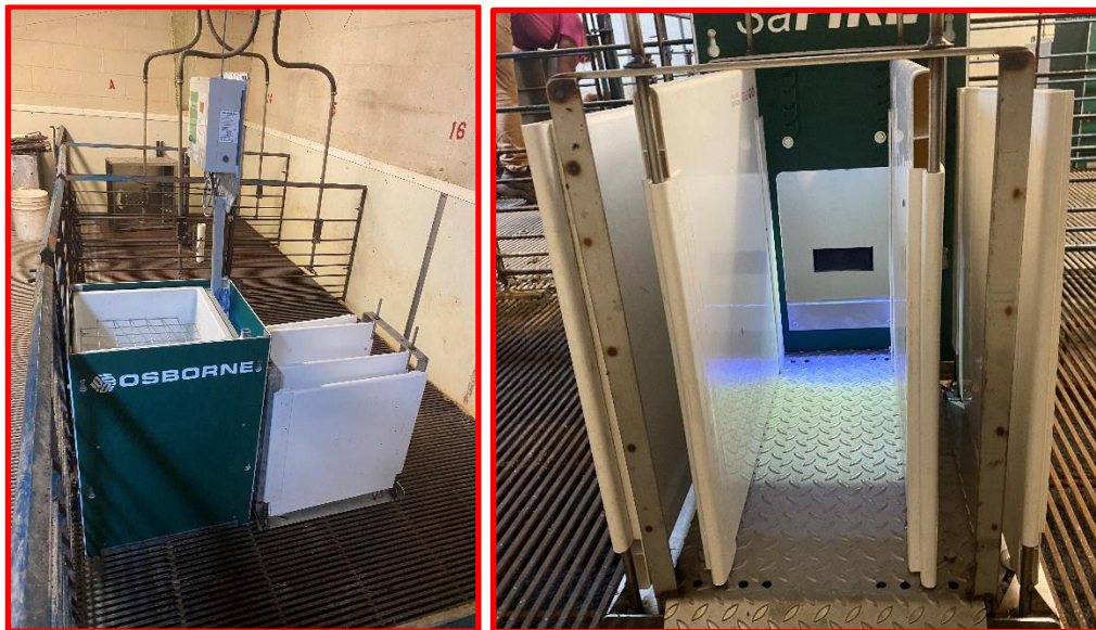
Figure 2. Small Animal Feed Intake Recording Equipment ( saFIRE ) recently installed in a nursery room at the Tidewater AREC in Suffolk. Panels that can be adjusted as pigs grow, limit access to the feeder to a single animal at a time. Each pig is fitted with an ear tag containing a transponder that identifies the pig and allows real-time collection of body weight and feed consumption data.
