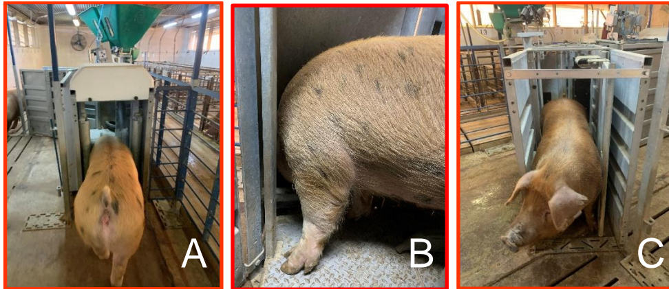
Figure 1. Electronic sow feeder (ESF) that was recently installed in the breeding-gestation barn at the Tidewater AREC in Suffolk. Each sow is fitted with an ear tag that contains a transponder providing access to feed. Panel A shows a sow entering the feeding station. Once the sow places her head in the feed trough (Panel B), the rear gate closes automatically, preventing other sows from entering. A pre-determined amount of feed is slowly dispensed in the trough, allowing the sow to eat without competition from other animals. Note the scale platform shown at the bottom of Panel B. The sow is automatically weighed as she consumes her feed. As shown in Panel C, the sow has completed her meal and leaves the station through a one-way side door. The rear gate then opens, allowing the next sow to enter the station.
